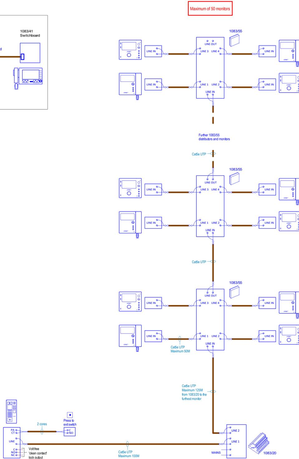
The maximum 'cable extension' or maximum total amount of cable in the 2Voice system is 800M.
