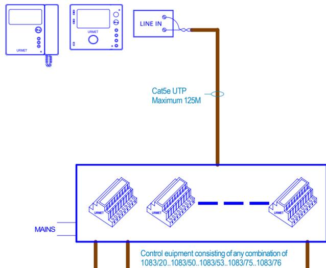
Control equipment consisting of any combination of 1083/20..1083/50..1083/53..1083/75..1083/76
