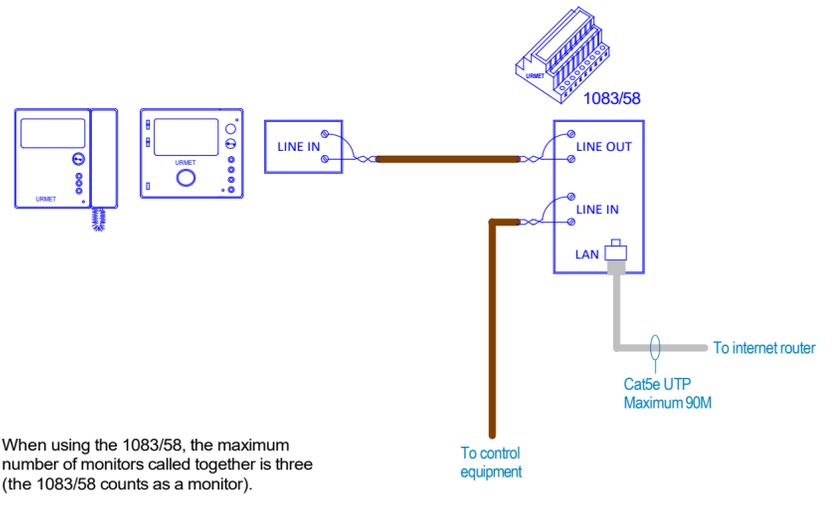
When using the 1083/58, the maximum number of monitors called together is three (the 1083/58 counts as a monitor).
