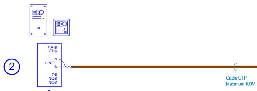
A maximum of 16 entry panels can be installed in this configuration
