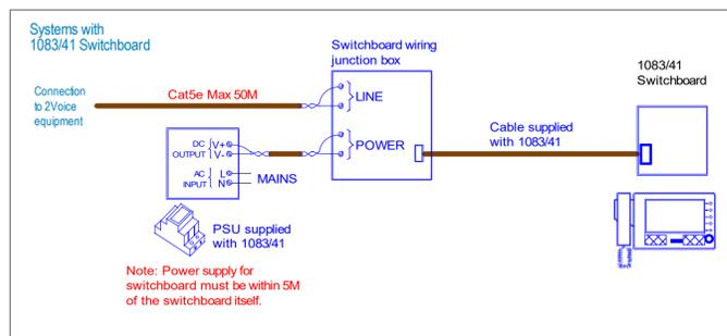
The maximum 'cable extension' or maximum total amount of cable in the 2Voice system is 800M.
