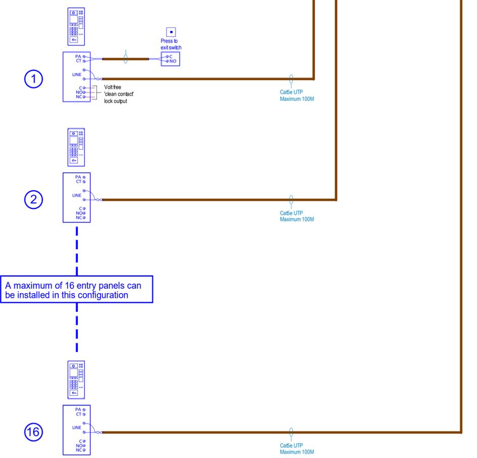
A maximum of 16 entry panels can be installed in this configuration
