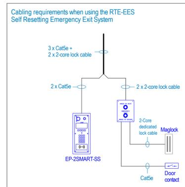
The maximum 'cable extension' or maximum total amount of cable in the 2Voice system is 800M.
