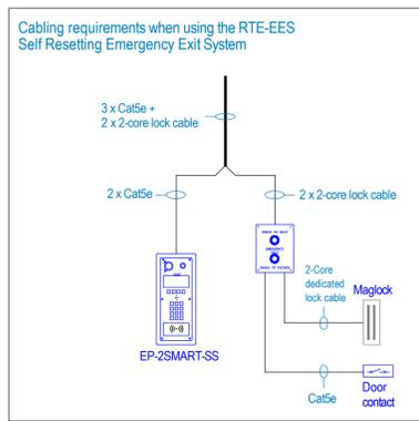
The maximum 'cable extension' for each section is 800M.
