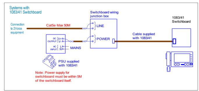
The maximum 'cable extension' for each section is 800M.
