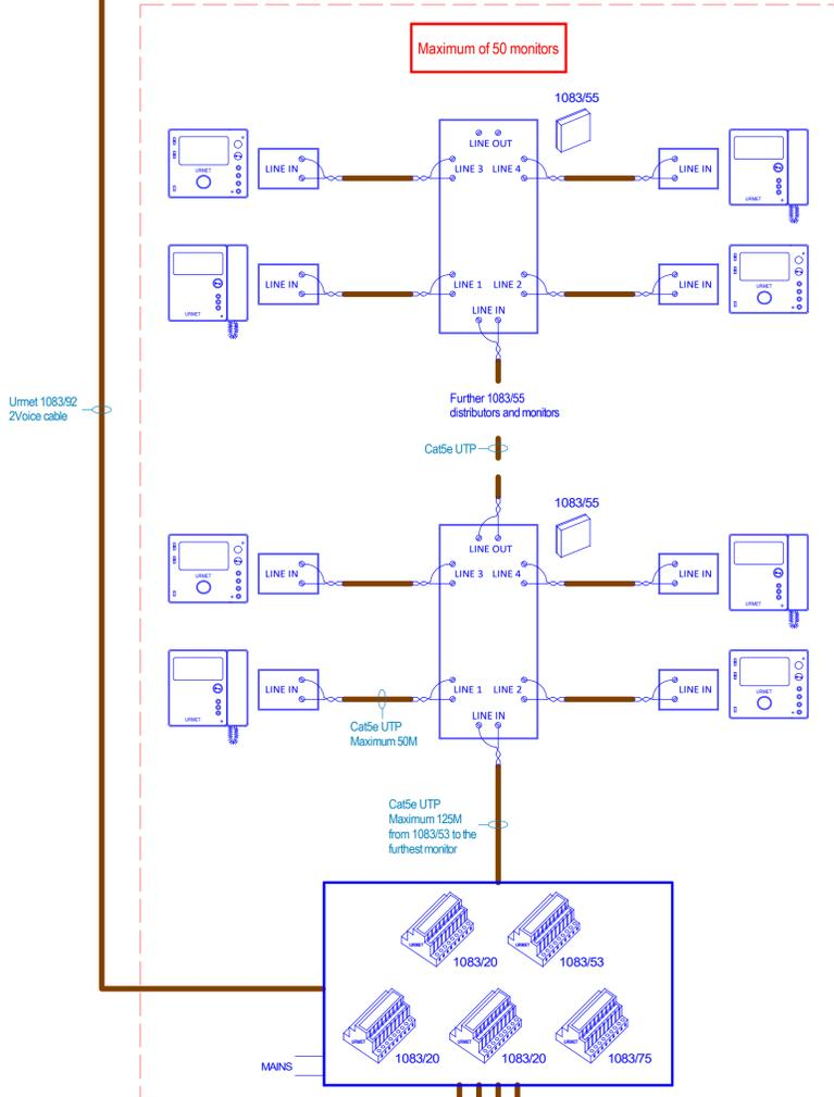
The maximum 'cable extension' for each section is 800M.
