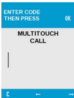
It is possible that when a number of buttons are pressed at the same time, a particular monitor or handset can be called, for example a caretaker's apartment.
