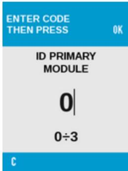
In a system with only one entry panel the ID is always **0**. In this case just press
