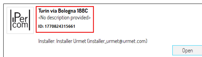
Figure 58: first check of site name and “Urmnet Cloud System ID” field
