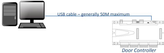
Used when a single PC is directly connected to the first controller to administer the site
